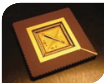
ABOVE: A novel device for trapping and controlling single atoms in the Laboratory of Schmidt-Kaler in Ulm. Milburn has developed theoretical schemes for simulating physics in these devices.
