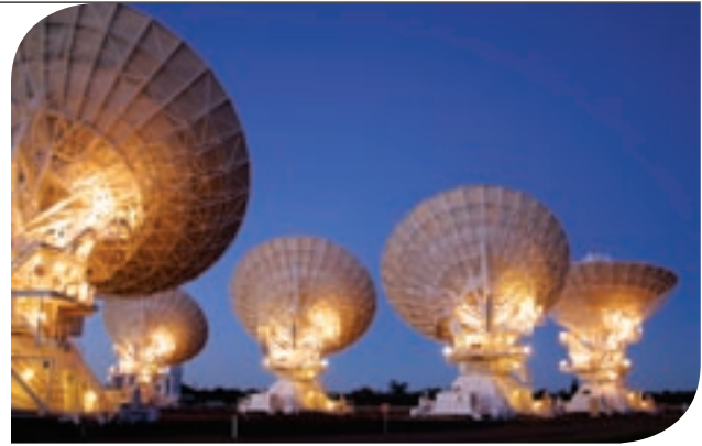
The Australia Telescope Compact Array has been equipped with sensitive receivers enabling it to detect radio waves as short as 3.5 millimetres. The new receivers incorporate special CSIRO-designed chips, made of the high-performance material indium phosphide. The new systems mean that the Compact Array will be the only set of telescopes in the southern hemisphere operating at these short wavelengths until the Atacama Large Millimetre Array telescope in Chile becomes operational at the end of this decade. Photo by: David Smyth, Source – CSIRO Division, Australia Telescope National Facility
