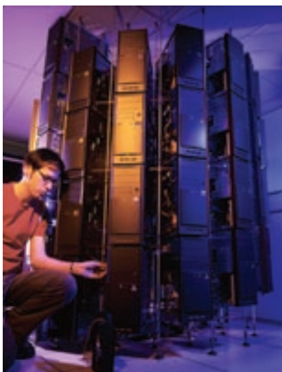
Caduceus – The Beowulf cluster ‘Caduceus’ used for the identification of novel drugs ‘in silico’. Photo by: Mark Fergus.
