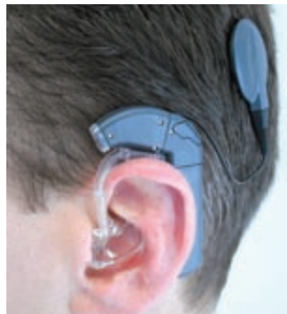
Picture of Audio Processor with earmould for Electric Acoustic Stimulation (the use of a hearing aid and a Cochlear Implant together in the same ear) worn by user. Photo by: Zipfer.
