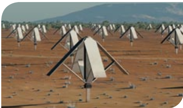
Sparse Aperture Array. © Copyright SKA: enquiries@skatelescope.org
