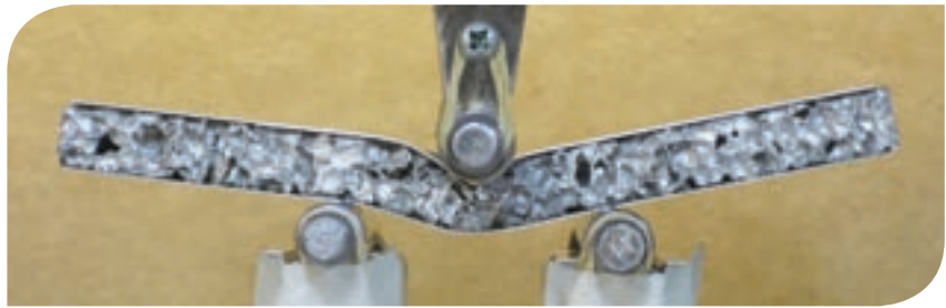
ABOVE: Asymmetric failure mode in three-point bending of a foam-cored sandwich panel with a span length of 50mm.
